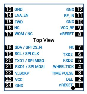
Figure 3-2 Pin Assignment
